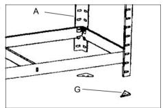
12. We recommend that the shelvng be secured to an adjacent wall using typical wall insert plugs and screws (not supplied) aligned with the assembly slots in the posts.
